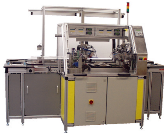
customer specific production center with BOSCH-Conveyor-System and 2 automatic soldering stations,
