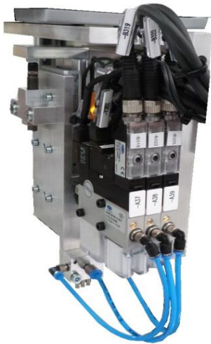
complete grippers with vacuum generators and Z-stroke
