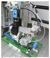
Economic A400L 4 axis (XYZT) IPC with WinControl compact laser control unit single optic SolderWireFeeder with Controller
