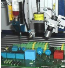
Economic A400L 3 axis (XYZ) IPC with WinControl compact laser control unit single optic external camera SuperSIGMA Dispenser Z-stroke for Dispenser
