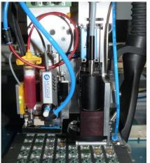
Economic A400L 3 axis (XYZ) IPC with WinControl compact laser control unit single optic external camera AeroJet with Controller ThermoController
