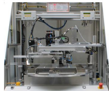
S1: Loadin / Unloadin S2: fluxing (X) S3: preform assembly (X) S4: Induction soldering
