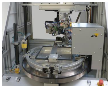
S1: Load / Unload S2: Scanner and MES S3: soldering iron (XYZ) S4: AOI
