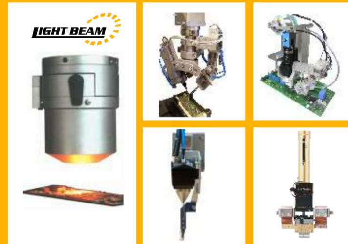
The soldering system LightBeam operates with IR-light focussed by convergence mirrors and optics. The heat radiation produces the temperature that is required at the Soldering Point. The energy can be regulated very exactly. Thus the light soldering is suitable in particular for the selective reflow-soldering.
